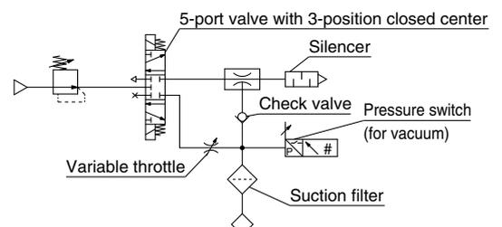
5-port valve with 3-position closed center is used to control the vacuum generation and release. A check valve is installed to the vacuum port to prevent vacuum pressure from being reduced when the supply valve is OFF\*1. A pressure switch is installed in the vacuum circuit to detect pressure. A suction filter should be mounted to the position where the duct collected by release air can be flushed by released air.
