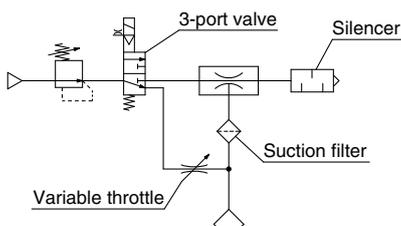
Power failure is prevented by changing the valve piping of Ex. 2 and applying vacuum generation N.O. specification. Variable throttle and suction filters are installed. A silencer is mounted to the exhaust port (to reduce exhaust noise).
