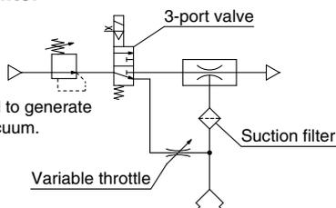
3-port valve is used to generate and stop the vacuum (vacuum release is performed simultaneously). Variable throttle is installed for break flow adjustment. A suction filter is protecting the ejector.
