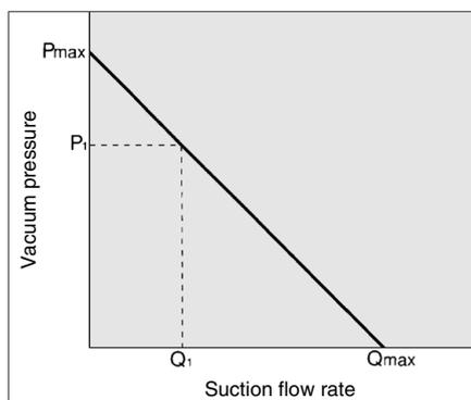
Flow rate characteristics are expressed in ejector vacuum pressure and suction flow. If suction flow changes, the vacuum pressure will also be changed. Normally this relationship is expressed in ejector standard operating pressure use. In the graph,  $P_{max}$  is maximum vacuum pressure and  $Q_{max}$  is maximum suction flow. The values are specified according to catalog use. Changes in vacuum pressure are expressed in the below order.
