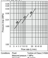
Measured pressure: 1 MPa Viscosity: 45 mm²/s Filter material: Paper Nominal filtration: 10 µm
