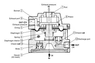
When the exhaust pressure from the switching valve enters into port ⑦, the piston ® and diaphragm ⑥ compress and displace spring (4), the exhaust pressure is released into the atmosphere from exhaust port (9), and at the same time the diaphragm is returned to its original condition by the recovery power of the spring.
