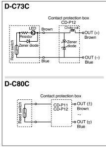
Note 1) Operating load is an induction load.
